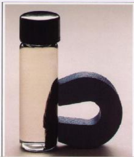
Left: Magnetic fluid is used in AR's mid- and high-range drivers for its excellent heat-transfer properties. It acts like the coolant in a car's radiator to protect voice coils against overheating. Opposite: Left to right, the AR38 s, AR28 s, AR18 s, AR48 s. Portrait, oil on canvas by Wenzler, reproduced courtesy of J.N. Bartfield, New York.
